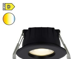
Rosalee 1-Kit 2410200103 Black | Aluminium | LED Module 7W 600lm | 2700K/3000K/4000K H: 4,2 cm | Ø: 8,6 cm
