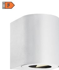
Canto 2 49701001 White | Aluminium LED Module 10,6W | 500lm | 3000K H: 10,6 cm | W: 8,7 cm
